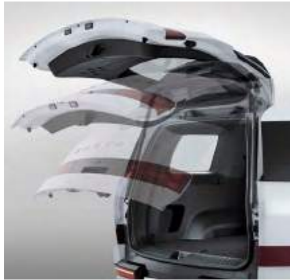
Smart Power Tailgate (Height Adjustable)
