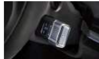
Column-type Shift by Wire (SBW)
